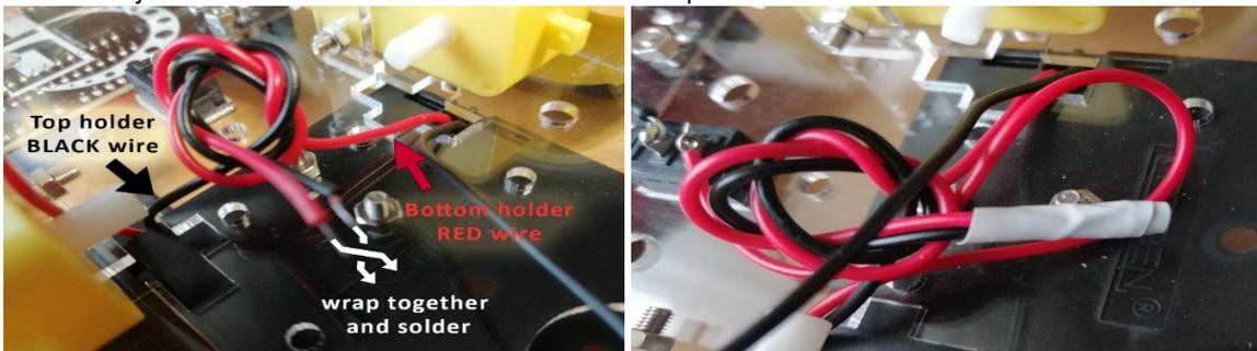
**Step 13) Solder the RED wire from bottom holder to switch**
