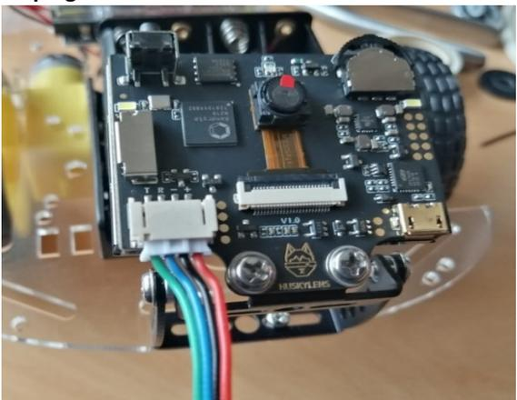
**Step 21) Pull the camera cable through the hole**
