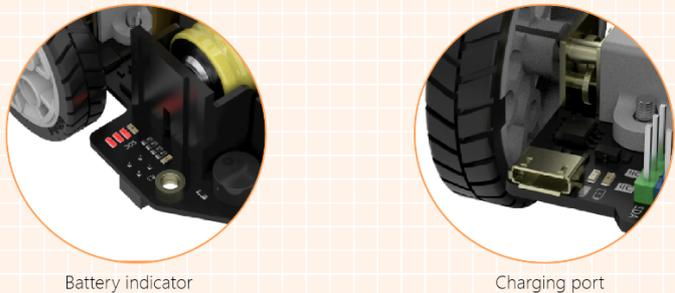
When the battery is fully charged, all LEDs will be on. The LEDs will turn off one by one as the power gradually decreases. If all lights go out, the battery needs to be recharged. Use your phone charger and connect it to charging port.
