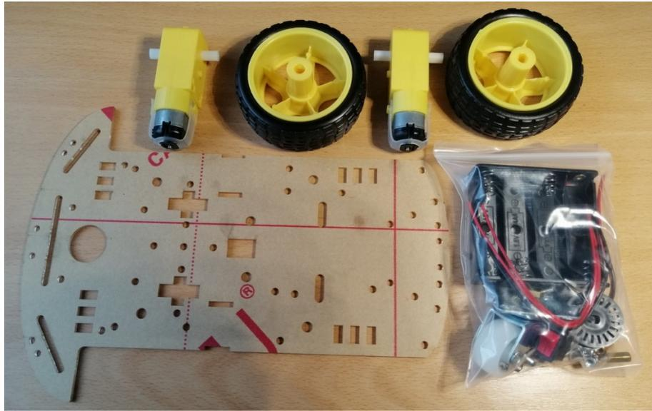
**Step 3) Peel off the protective paper from the big board and motor brackets**
