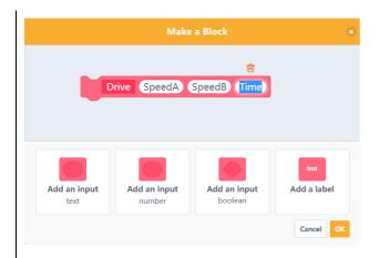
Basic idea is to get SpeedA and SpeedB values (acceptable range: -255 to 255), check if any of it is negative (or both) and if it is - reverse the direction by setting the correspondent direction pin. But to drive the motor you have to use the absolute value on PWM pin..
