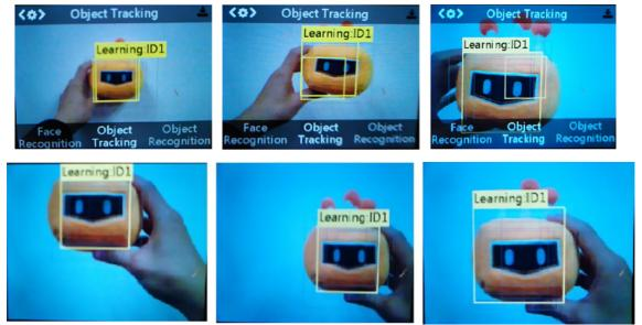
When HuskyLens can track the object at different angles and distances, then release the "learning button" to complete the learning. If there is no orange box on the centre of the screen, it means that the HuskyLens has already learned an object. If you want to track another object - select "Forget Learned Object" and learn again.
