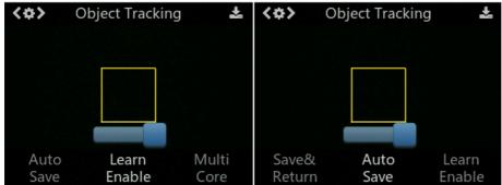
When restarting HuskyLens, the last learned object is not saved by default, and you can turn on the switch to save models automatically.
