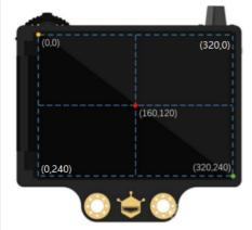
The coordinates of the object centre point obtained through the program are also within this range. For example, if the coordinate values obtained are (160, 120), the object being tracked is in the centre of the screen.
