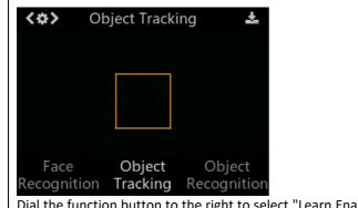
Dial the function button to the right to select "Learn Enable", then short press the function button, and dial it to the right to turn the "Learn Enable" ON, that is, the square icon on the progress bar is turned to the right. Then short press the function button to confirm this parameter.
